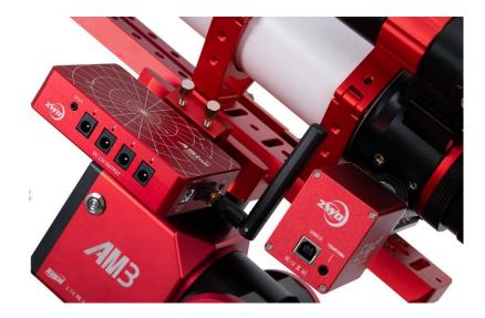
Step 3: Power on your ASIAIR and AM3. When the system of the ASIAIR is ready, select the corresponding ASIAIR wireless signal in the wireless LAN of your smartphone.
