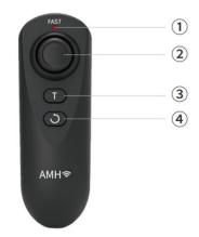
(1) Light Indicator: Indicates the High or Low Slew Rate of the AM3. High Rate: when the red light is on.
